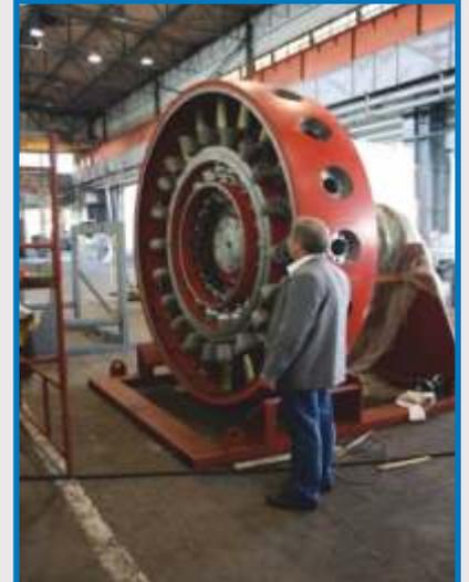
The fans are executed from carbon, high-alloy, acid resistant, heat-resisting steel as well as aluminium. Precision of co-acting fan parts is ensured by their detailed inspection at all manufacturing phases. Welded joints are tested by using magnetic-particle, penetrant, ultrasonic or radiographic inspections.
