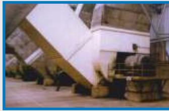
They are also used as general purpose fans in various technological processes to provide pressure increase up to 25 000 Pa.
