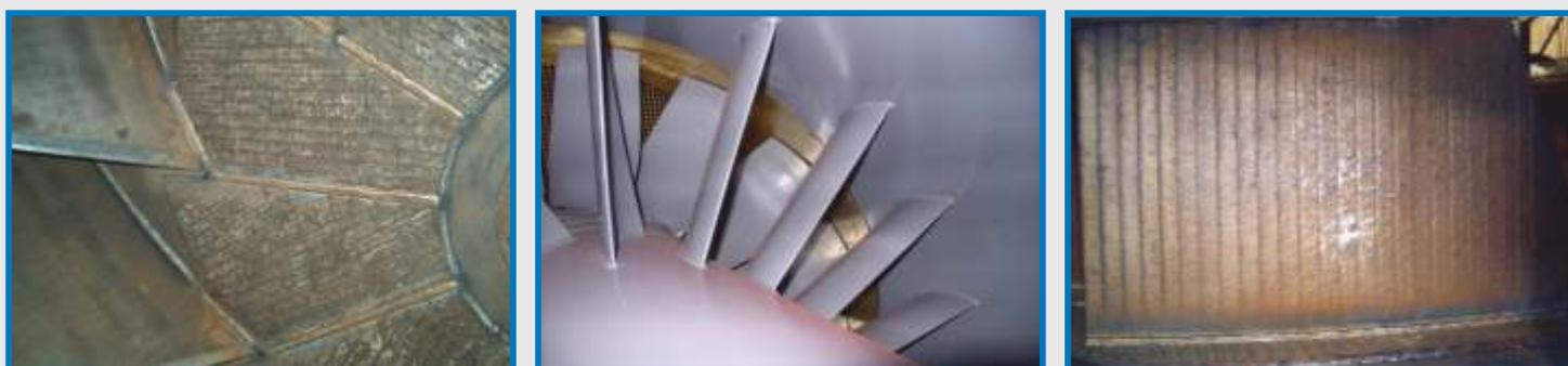
We use special linings, padding welds or anti-wear spraying which significantly elongate lifetime of fan parts. Furthermore such materials are suitable for temperature up to 600°C what allows to use these fans in a wide variety of applications.
